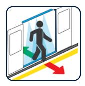
Sensors cover the entire door's width and are installed directly above the gap.
